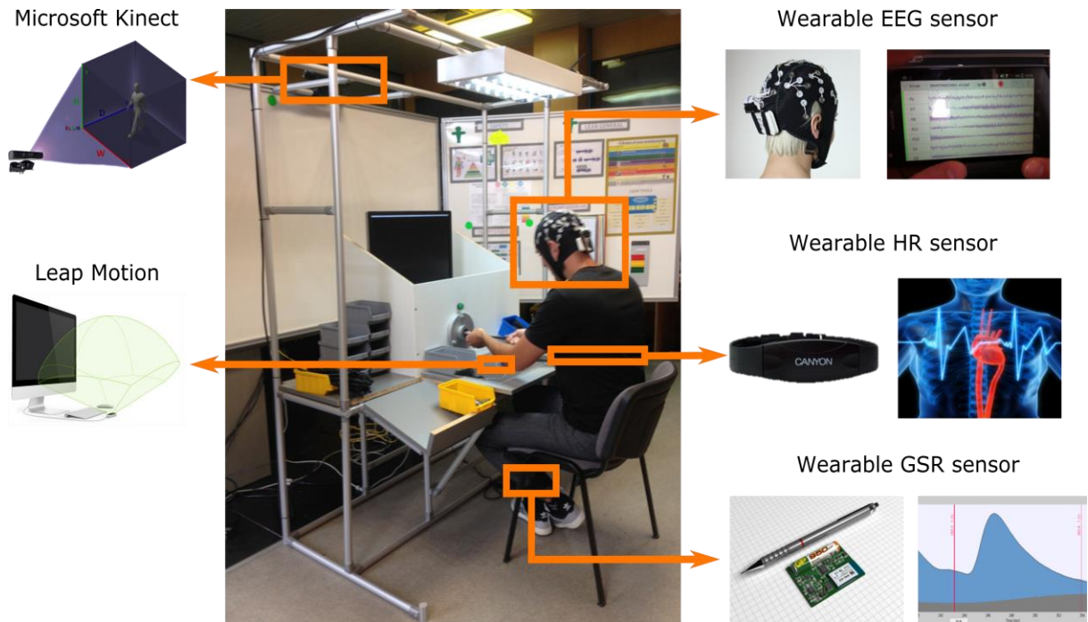
Figure 5-3: Figure 3. Replicated workplace and the sensors placements
