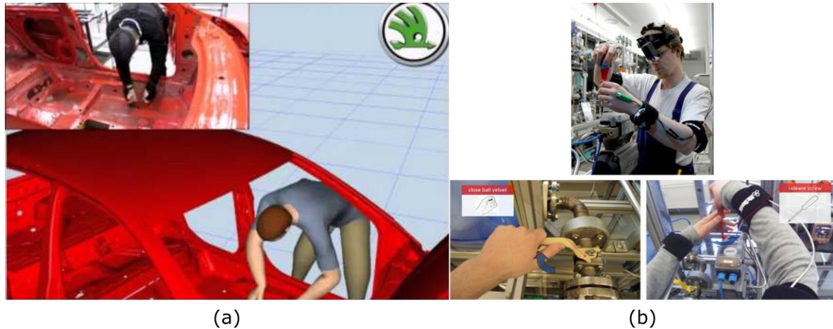
Figure 4-1. (a) Combination of Synertial IGS suit with Siemens JACK software for ergonomics evaluation of car assembly, a case study from Skoda automotive (adopted from: www.synertial.com ); (b) – IMUs sensor network developed on Cognito project. In this case, apart from possibility to track the workers motion, the Cognito system provides also support to the worker in sense of information on head-mounted VDU, as seen on figures bellow (adopted from http://www.ict-cognito.org )
