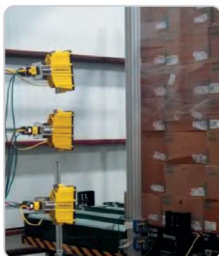
Cognex image-based readers can decode multiple codes over the width and height of the pallet, in any orientation.
